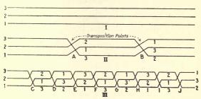
Fig. 106.—Transposition of three-phase circuits.
